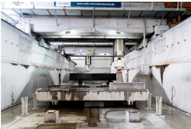
To process such blocks precisely, Reitz relies almost exclusively on machines developed and built in-house: four gantry-type milling machines and two 5-axis gantry machines, all controlled by Siemens 840D. To ensure safe, fast, and precise granite machining, the company uses Vericut simulation software.
