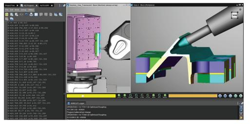
complex 5-axis closed wall barrel cutting toolpaths. It is also a great tool for training employees and sharing knowledge. The live simulation cut stock display in the software provides а way to visualise and demonstrate machining strategies and toolpaths to shopfloor machine
