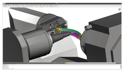
machine is capable of in a specific application before they buy. So, as already outlined, Starrag builds a bridge to the future by means of NC simulation: the customer's real NC program is checked for collisions etc. on the virtual machine in VERICUT. The real process is digitised on the basis of the NC program, with the help of the machining center's Digital Twin. Phillip Block, Marketing
