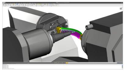
machine is capable of in a specific application before they buy. So, as already outlined, Starrag builds a bridge to the future by means of NC simulation: the customer's real NC program is checked for collisions etc. on the virtual machine in VERICUT. The real process is digitized on the basis of the NC program, with the help of the machining center's Digital Twin. Phillip Block, Marketing
