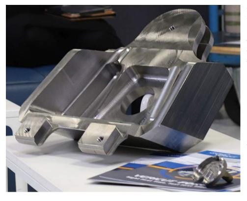
With the capabilities of VERICUT Force now proven to the engineering team at SECO the partners thoughts turned to the real value of applying it to actual customer components. Α forged 6AI-4V titanium aerospace component highlights the results as David Magnall explains: "We had already reduced the cycle time of the complex pylon bracket down to 4 hours, but just running it through Force reduced it down to 3 hours. which is iust phenomenal. It's not like
