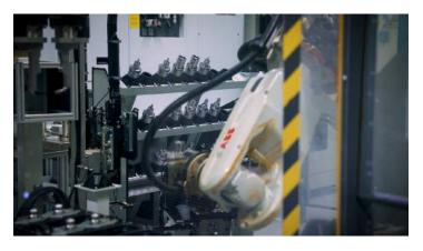
The Gimo site is up and running 8,760 hours per year and features extensive automation. In fact, the whole night shift is unmanned, operated by hundreds of industrial robots and automated guided vehicles (AGVs). Furthermore, a digital 'thread' runs throughout the factory that automates everything from customer order to despatch, with data feedback from production to the company's systems
