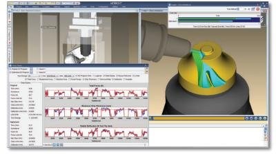
VERICUT is equipped with NC program optimization capabilities. Based on the cutting tool geometry, part material, and programmed cutting conditions, VERICUT automatically determines the optimum safe feed rate for each cut. The VERICUT optimized NC program will greatly improve cutter performance resulting in significant cycle time savings, reduced tool wear, improved tool life, and better finished parts.
