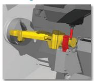
VERICUT simulates milling, drilling, turning, multi-tasking mill/turn, and EDM operations. Errors that could ruin the part, damage the fixture, or break the cutting tool are easily identified. VERICUT supports G-codes and native CAM files and includes analysis tools to measure and compare the cut part with the design model. You can model any cutter, fixture, or holder shape. During simulation you create in-process inspection instructions and export a CAD model of the "as-machined" part.
