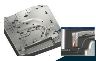
value as it is for the current material, HP4M mold steel, might not be suitable, so the optimization setting was set at 95% of the chip thickness value, which was obtained through the Force analysis. The 95% was selected based on CGTech's accumulated data and know-how through various past tests done by CGTech.
