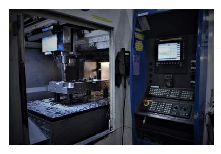
machining centers. "We were experiencing way too many collisions, mainly because of our deep cavities and big parts, some of which measure 30" x 40" across and up to 10" deep," he says. "We needed a way to protect our machines, and reduce the downtime and expense that comes with crashed spindles. For example, there've been instances where we replaced eight spindles in a single year, each one costing us a day or two of downtime, or even three to four weeks if a replacement
