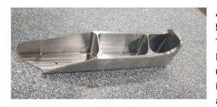
A Titanium (Ti-6Al-4V) part was machined using a 5-axis DMC-100U duoBLOCK to test the software. To machine a part faster and safer, FORCE cuts the NC code into small segments and applies the optimal feed rate for each segment, improving the efficiency of the toolpath and eliminate any risk due to
