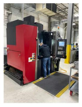
centers, most with four or five-axis capabilities. The EDM department houses Makino wires and sinkers, the largest with nearly 20-inches of Z-axis travel. Automated coordinate measuring machines (CMMs) and vision systems from Hexagon and Micro-Vu are located in strategic locations. All equipment is arranged in cellular configurations for the greatest efficiency.
