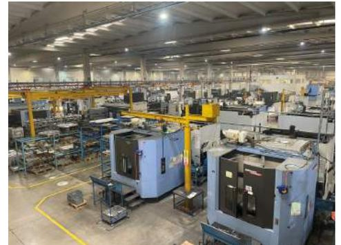
“With over 80 high-technology CNC machines we’re able to produce complex and precision parts from all kinds of light and hard metals, including aluminum, steel alloys, stainless steel, titanium, magnesium and nickel-based superalloys from plate, sheet, castings and forgings in compliance with customer specifications,” explains Onur Benzergil, New Part Supervisor at HMS Makina.
