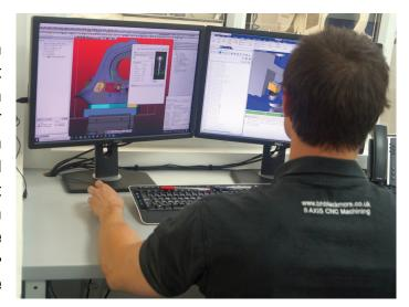
Lead CNC Programmer, Jan Plovucha, was a catalyst for the application of VERICUT at Blackmore Precision Engineering. For CAD/CAM the company uses Open Mind's HyperMILL software which has a direct interface with VERICUT to import all of the necessary detail including the Lang high pressure clamping system and zero point plates used across the shopfloor. The goal is to 'hit' the component in one using the experience of the programmers to achieve this.
