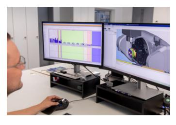
Vericut Force is a physics-based optimisation module that calculates cutting parameters not generically, but based on real material properties, tool specifications, and machine dynamics.
