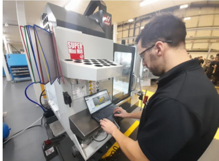
"Learners are introduced to CNC via absolute and incremental programming, programming point-to-point and learning about sub routines, tool changes, safe moves and so on," explains Jake. "Typically, the learners begin by machining simple 2D profiles from plastic or aluminium, working towards assessment tasks. For milling, these assessments might include profiling, chamfering, pocketing, drilling and CAM cycles, for example."
