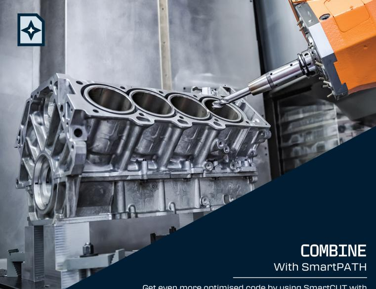
Get even more optimised code by using SmartCUT with SmartPATH, detecting the start point and end points of air-cut segments and computing the fastest path to the start of the next cut.
