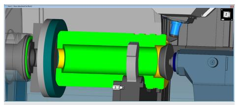
Enhanced Sectioning allows the NC programmer to inspect the inside of a part during simulation. This unobstructed view will help identify any potential problems with the workpiece and machine tool.
