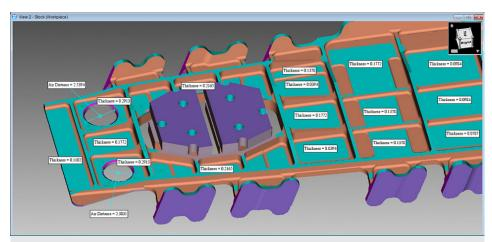
X-Caliper dimensions are easily displayed on the part. Measurement labels can be adjusted for optimal viewing. Multiple dimensions are able to be displayed and referenced in VERICUT reports.
